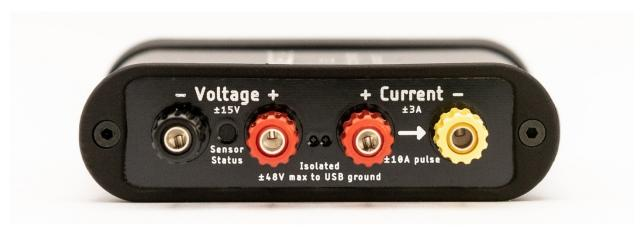
Your JS220 measures the voltage across the Voltage + and Voltage – binding posts. Your JS220 measures the current flowing through the Current + to the Current – binding posts. If you have a power source and target device, connect the positive side through the current binding posts. You can then connect the voltage signals across either your power source or your target device. For more connection examples, see Section 9.
