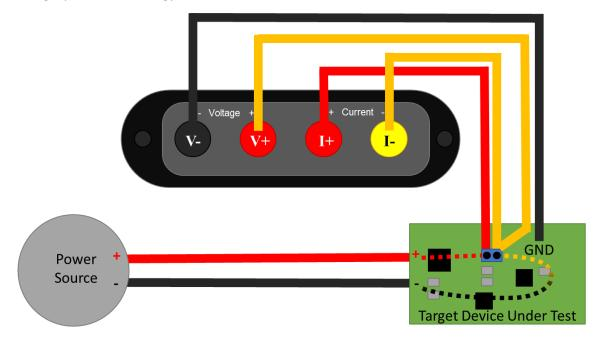
This connection recommendation shows a Kelvin-style 4-wire connection, which helps improve accuracy and minimize noise pickup. Connect the JS220 using two wire pairs, one to measure current and one to measure voltage. Twist the insulated V+ and V- wires together and the I+ and I- wires together to further reduce noise pickup. For less accuracy and perhaps a quicker setup time, connect V+ to I+ and V- to PS-.
