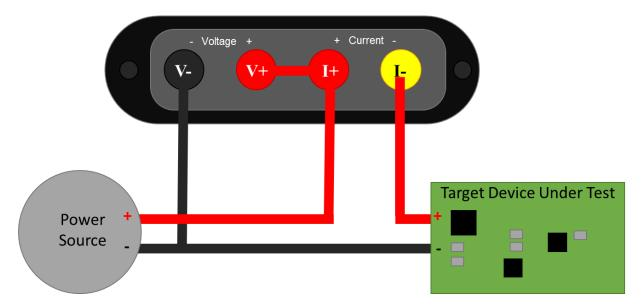
Note that the V- wire is connected to PS- and T-. It does not connect to PS+. This setup configures the Joulescope JS220 in high-side current sense configuration.
