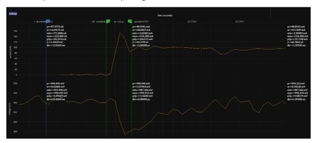
This test shows the current consumption going from 97 nA to 100 mA. The JS220 responds immediately to the change in current. The very slight ripple before the edge is caused by the low-pass FIR filter on the JS220.
