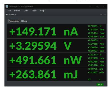
To measure the current and charge, connect the Joulescope **Current** port inline between the positive output from your power source and your target device under test. The maximum voltage between any port **Current +**, **Current -**, **Voltage +**, and **Voltage –** should never exceed ±15V. All sensor ports are electrically isolated from USB, but the voltage between any port and USB ground should never exceed ±48V.
