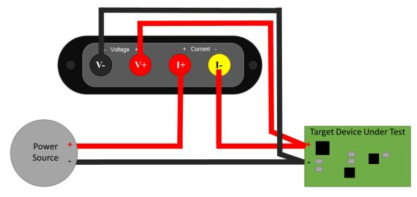
To minimize noise pickup, you want to minimize the loop area. The easiest way to do this is twist the insulated + and - wires together from PS+ and PS- all the way to T+ and T-, like this
