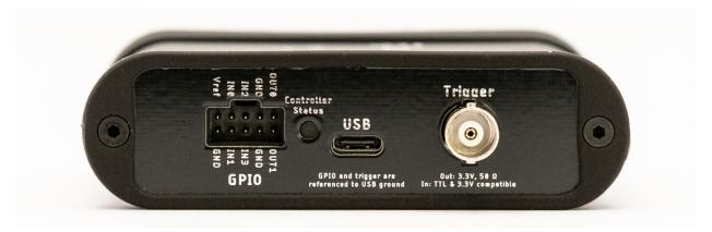
Use the provided USB C to USB A cable to connect the USB host computer connector to your host computer. If your computer only has USB C ports, use an adapter (not provided) or a USB C to USB C cable (not provided).
